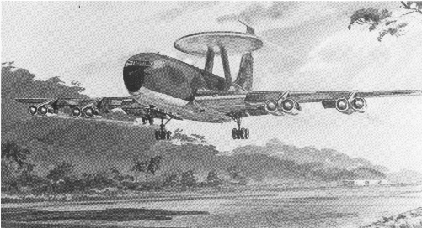
AWACS. Eight-engine version of Boeing 707-320 shown with large radome designed to house surveillance radar antenna. AWACS fleet would serve as an Airborne Warning and Control System, for both tactical and air defense forces.
